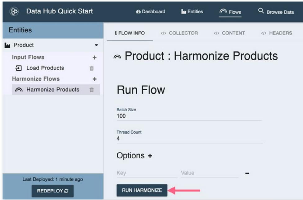
Figure 3: This screen capture from the Data Hub Framework illustrates the organization of flows for various entities on the left, and the operations, job tracking and transform step management on the right.
